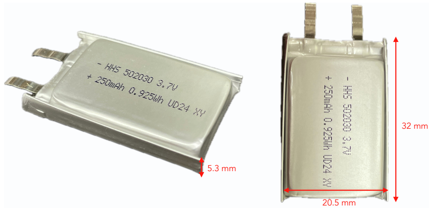
Figure S1: 502030 pouch cell used in this study, annotated with its dimension.
