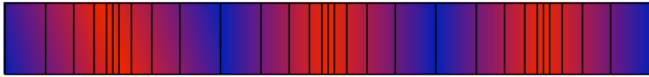
(a) Longitudinal wave propagation. Here, each bar can be thought of as representing a single particle (or a fixed number of particles), and all particles are oscillating horizontally. Hence, regions with higher densities of bars correspond to higher pressure values.
