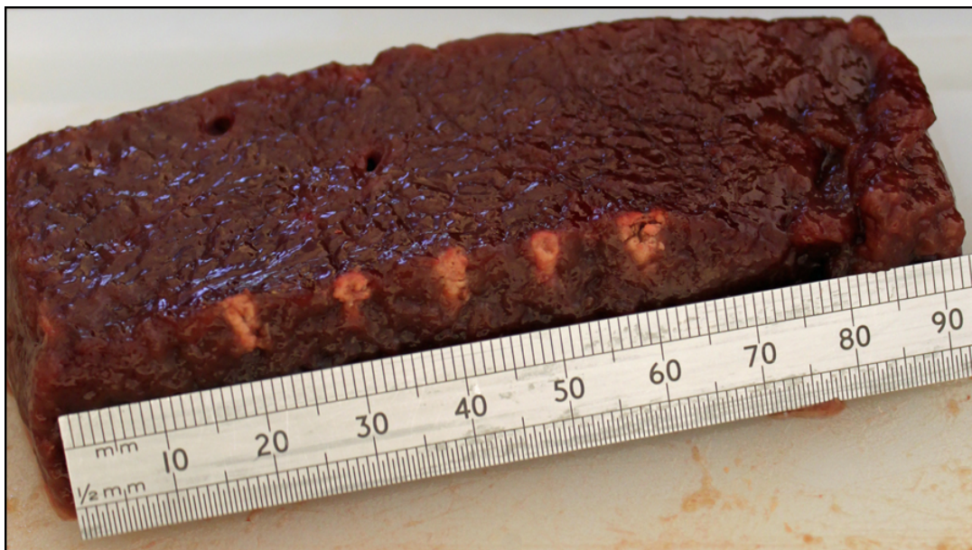
(b) Axial view of the 5 s lesions (the rightmost column in the grid of Figure 6.2a). Only the distal half of each lesion (2 cm to 4 cm deep) is shown in the image.
