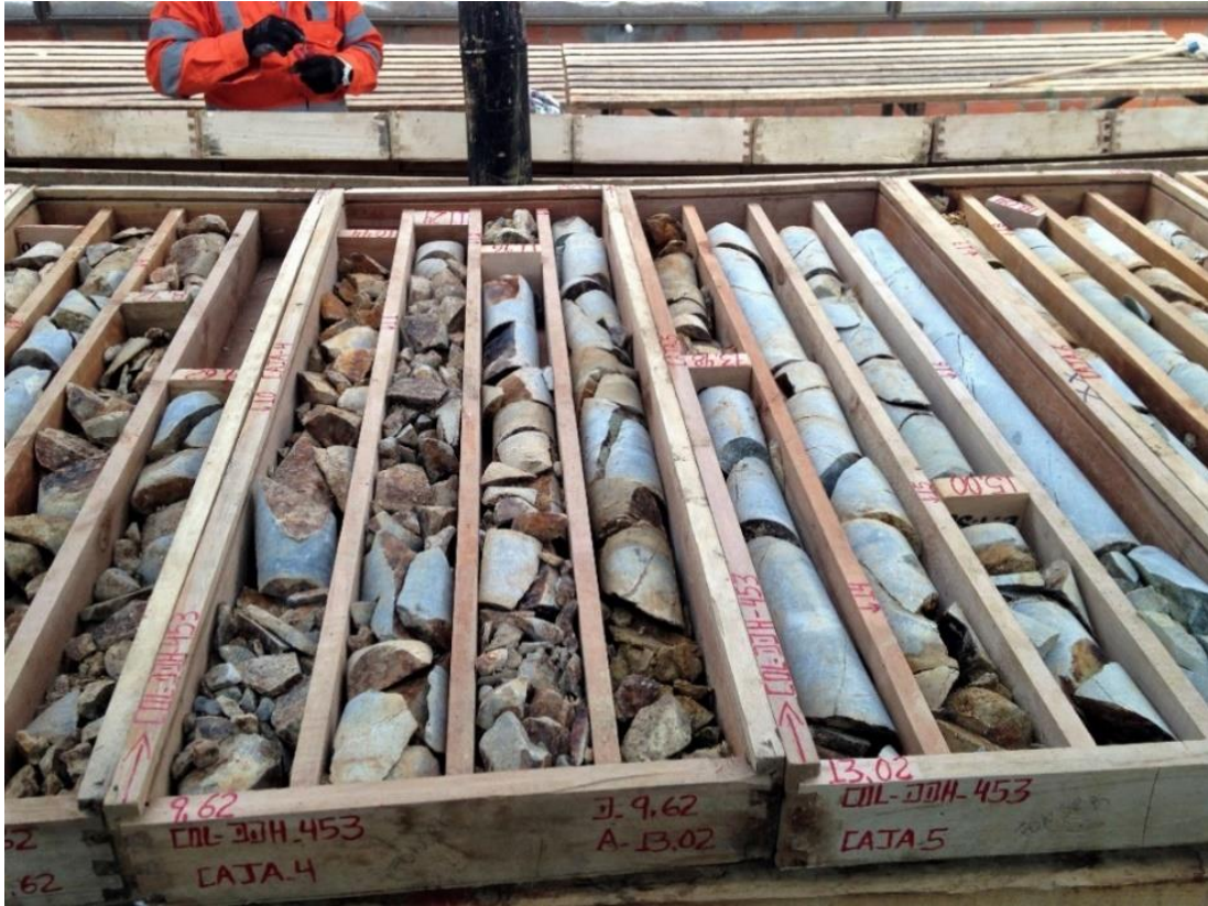
2.2 Rock samples from the drilling programme at La Colosa, displayed to visitors of the mining site at the repository where they are catalogued and stored.
