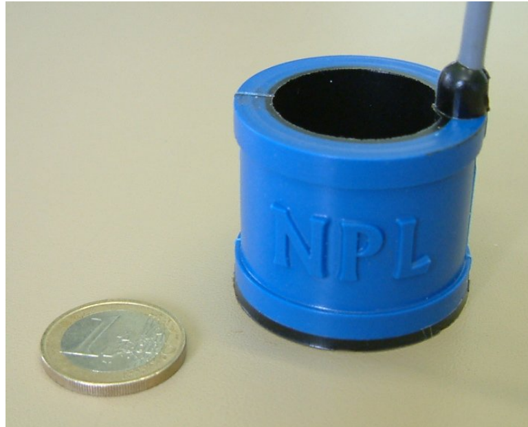
Figure 5.1: The National Physical Laboratory Cavitation Sensor (NPLCS). The prototype, three-dimensional cavitation sensor was based upon an extension of this design, incorporating multiple elements to achieve three-dimensional mapping of the cavitating field.
