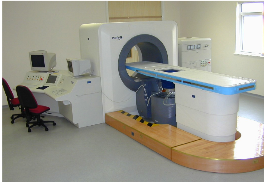
Figure 1.3: Illustration of the Chongqing clinical HIFU device in use at the Churchill Hospital, Oxford. The HIFU transducer is positioned below the central table, on which the patient lies, and is aligned using a computer-controlled, motorised positioning system. Acoustic coupling with the patient is achieved via a pool of degassed and deionised water, whilst treatment monitoring is limited to B-mode hyperecho. Image courtesy of the Oxford HIFU Unit.
