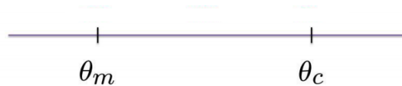
Figure 1.4: For nematics in general, when \theta < \theta_m , the material is in other liquid crystal or solid phase; \theta_m < \theta < \theta_c , the material is in nematic phase; \theta > \theta_c , the material is in isotropic phase, where \theta_m and \theta_c are some threshold temperatures in phase transitions which depend on the given material.
