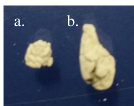
Figure 4.8 The two types of polymer morphology produced with a graphite additive, a. agglomerations on small elongated particles not containing graphite, b. large masses with encapsulated graphite visible through the surface cracks
