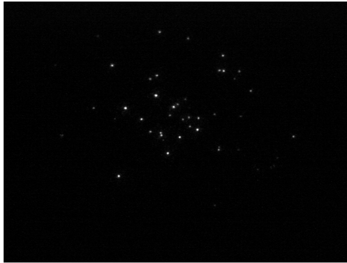
Figure 3.5: Ion image taken of signal from a single laser shot. Each flash on the screen is shown over an area of pixels approximately 2 mm in diameter.
