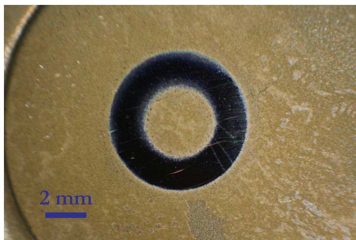
Figure 6.1: Optical image of CHCA sample prepared for imaging with a fast detector.
