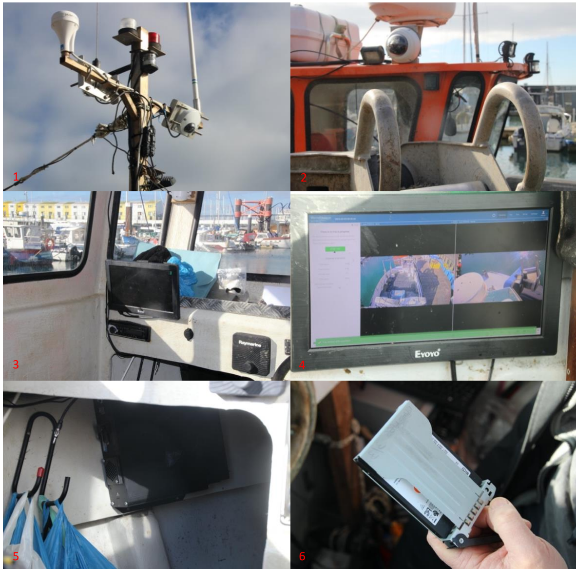
Figure 14 - 1. A GPS unit (left) and camera (right) mounted to the vessel mast. 2. Camera facing the net hauling. 3. System display houses in the wheelhouse. 4. System display showing both camera angles. 5. Computer stowed beneath the dashboard. 6. Swapping hard drives. Author’s images.
