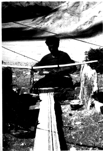
32. A gauge rod ( sug-lcags ) is used in pile weaving, and the knots are made around this.
