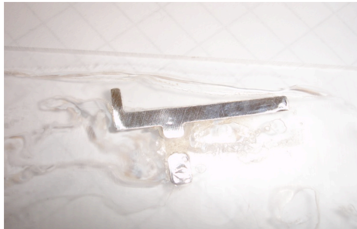
Figure 2-2 Polished section of a retrieved and sliced tibial component. The section has undergone radiography and has been prepared with a pre-stain.
