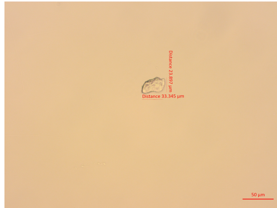
Figure 4.14: Single dig in one of the quartz coupons, visualised at the microscope with a magnification of 20\times .
