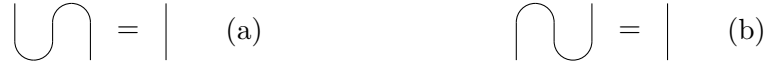
Figure 2.12: The snake equations in a graphical language that is read from bottom to top, e.g. the ZX-calculus.
