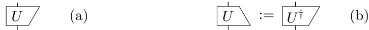
Figure 2.13: (a) Graphical representation of a map with one input and one output in a dagger category. (b) The dagger of a map is denoted by an upside-down version of the asymmetrical box.
