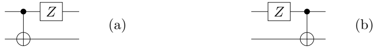
Figure 2.15: (a) A controlled-NOT gate, followed by a Z-gate on the control qubit, and (b) a Z-gate followed by a controlled-NOT gate.
