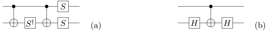
Figure 4.1: Two quantum circuit decompositions for the controlled-Z operator in terms of controlled-NOT and single-qubit gates: (a) using phase gates and (b) using Hadamard gates.
