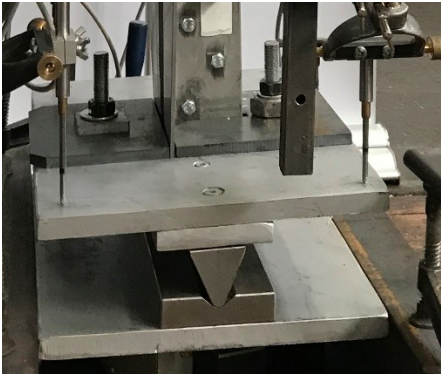
Fig. 5 Boundary condition at the bottom of the built-up T-section column — knife-edge devices and steel clamps (all dimensions in mm).
