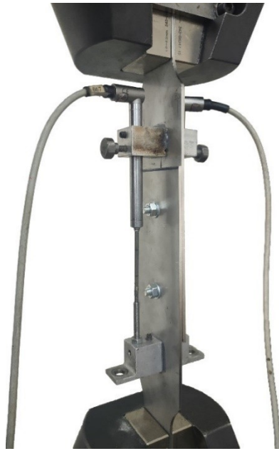
(a) Single lap shear test set-up
