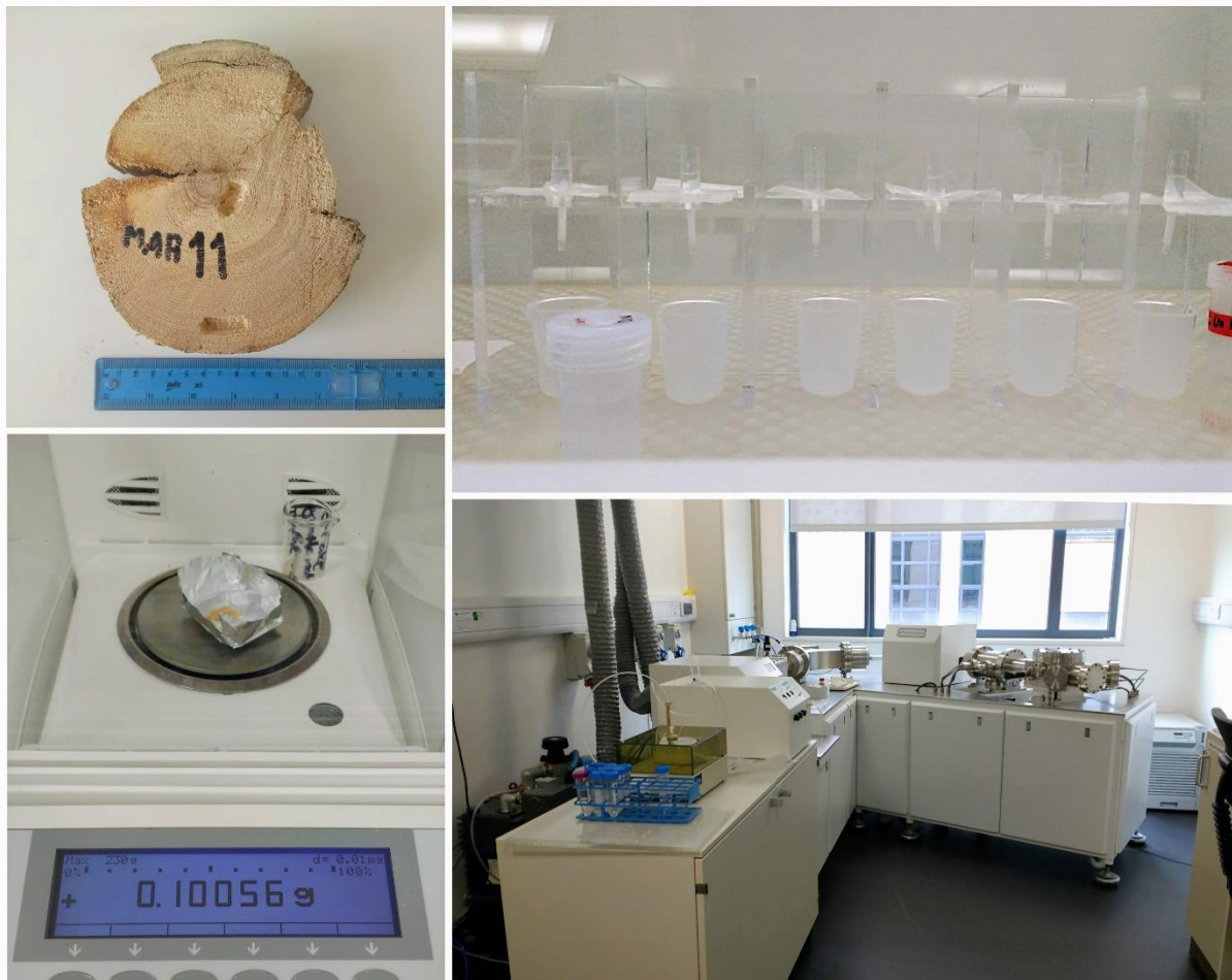
Figure 2.6. Subsample extraction of wood shavings, geochemical column-chemistry for strontium extraction and analysis via MC-ICP-MS.
