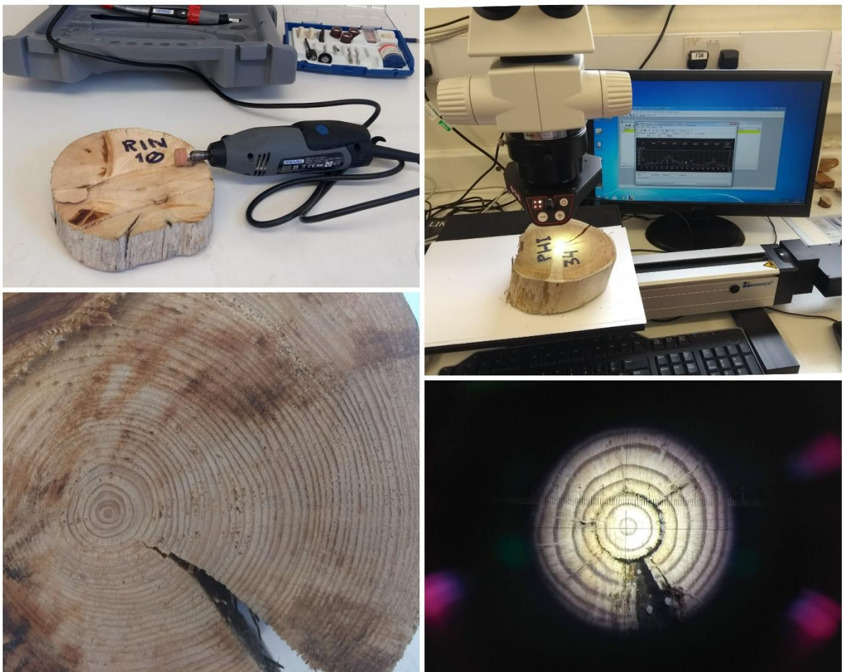
Figure 2.4. Preparation steps for driftwood samples for tree ring width analysis with LINTAB tree-ring measurement table and TSAP-Win Professional version 0.89 (Rinn, 2011) for dendrochronological crossdating.
